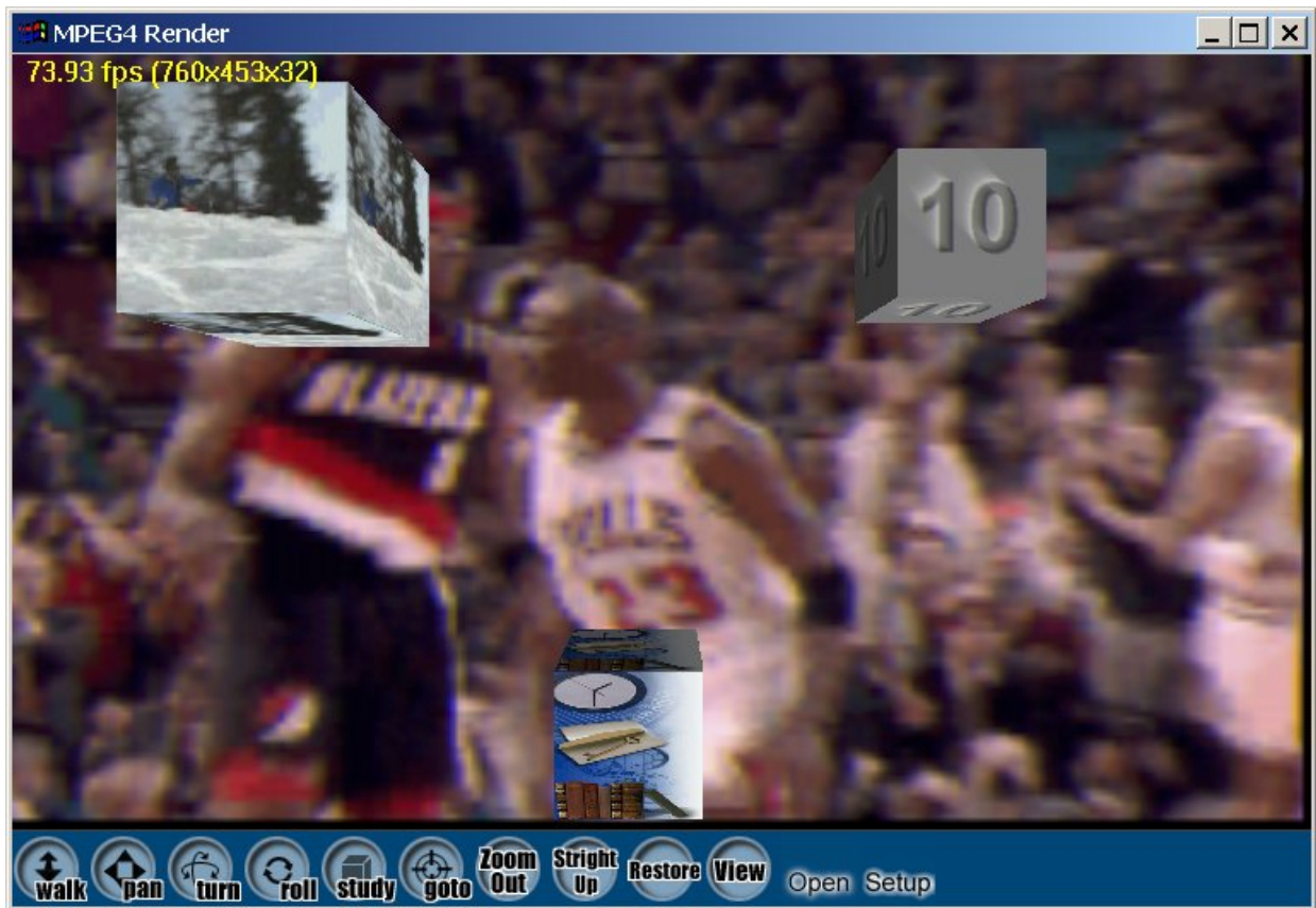
Figure 7: Snapshot of the rendering module, which is integrated with other modules to show 3D nodes. In this picture, there are three moving cubes with each face containing a video, and the background texture is also a video object. The average performance is about 70 fps.
